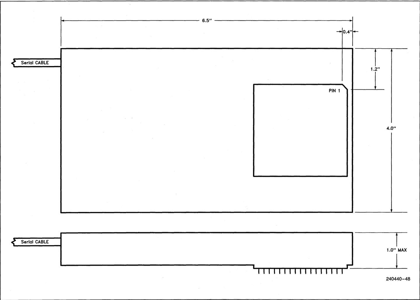
Figure 13.4a. ICD-486™ Probe Dimensions
