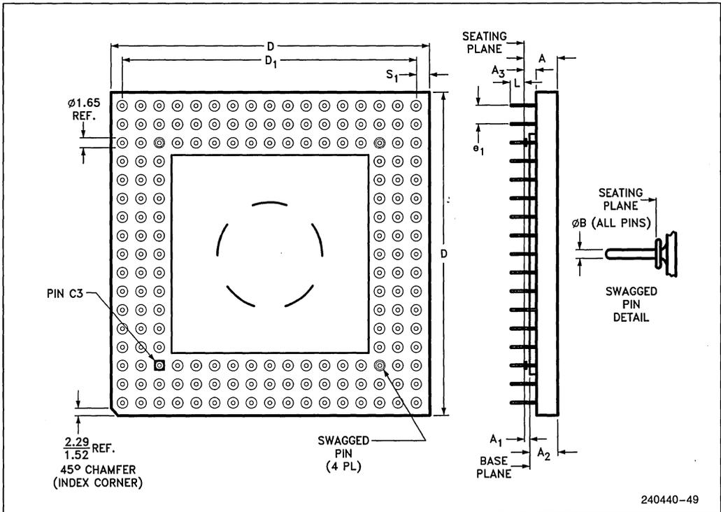
Figure 14.1. 168 Lead Ceramic PGA Package Dimensions
