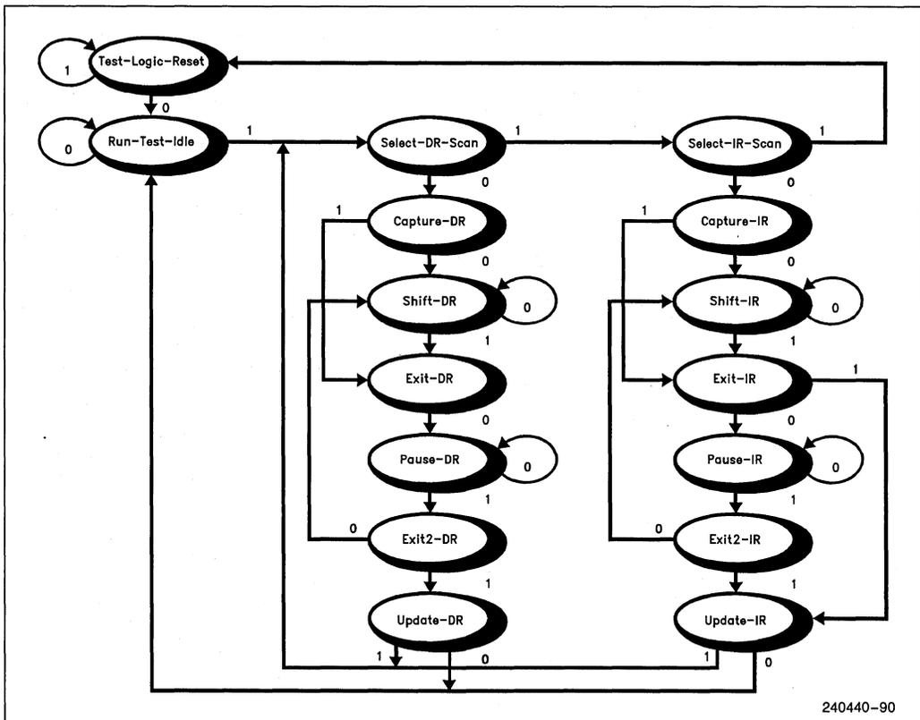
Figure 8.3. TAP Controller State Diagram
