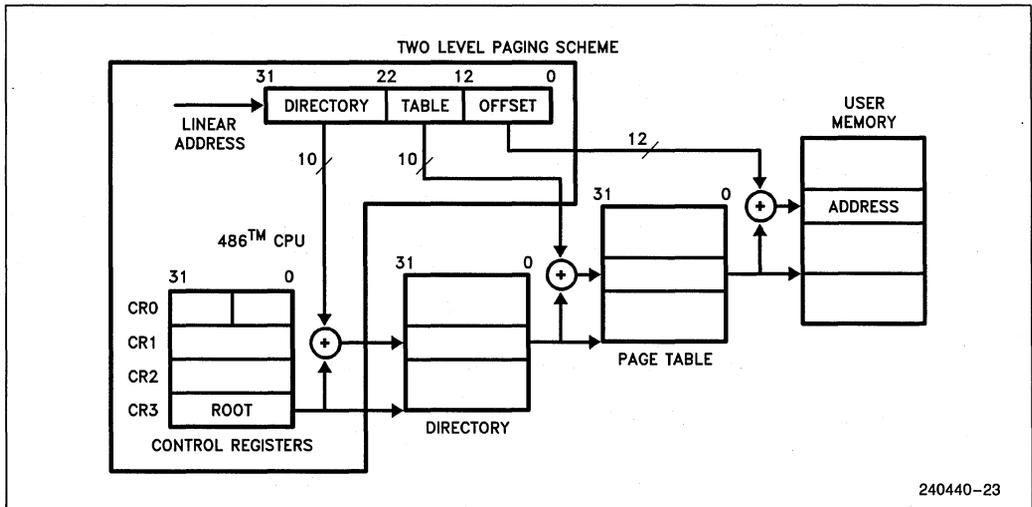
Figure 4.19. Paging Mechanism
