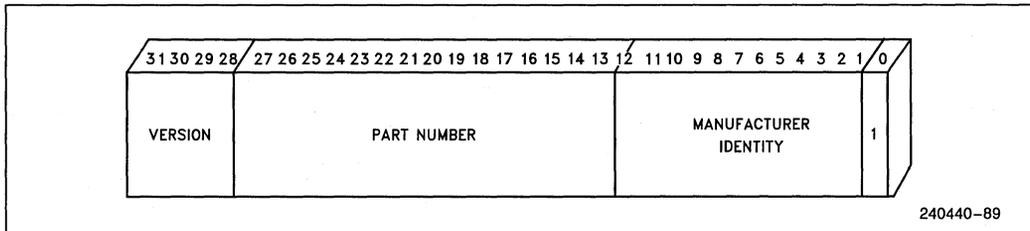
**Figure 8.2. Format of Device Identification Register**
