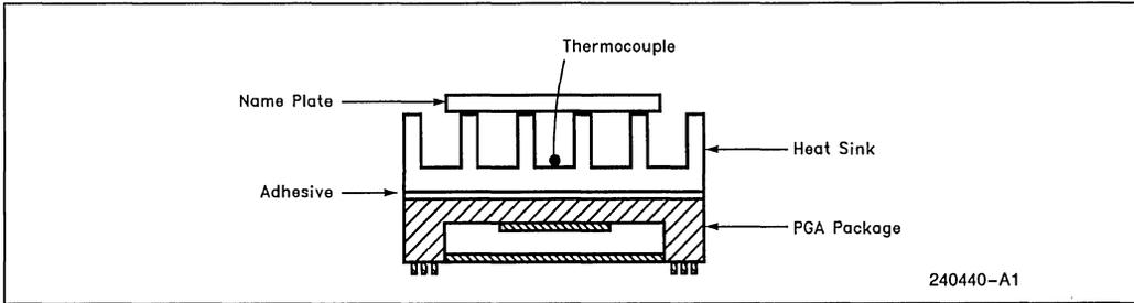
**Figure 12.5. Heat Sink Measurement (0.0005" Dia. Thermocouple) on the Center of Heat Sink with a 90° Angle Adhesive Bond Through a Hole Drilled Through the Center of the Name Plate.**
