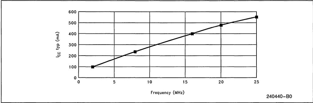
Figure 15.6. Frequency vs I<sub>CC</sub>(typ) (PGA Version)
