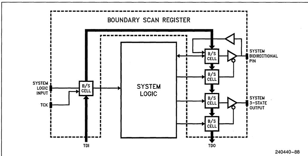
Figure 8.1. Logical Structure of Boundary Scan Register
